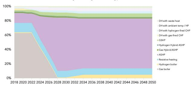
Figure 21: Non-Domestic New Building Heating Technology Mix
